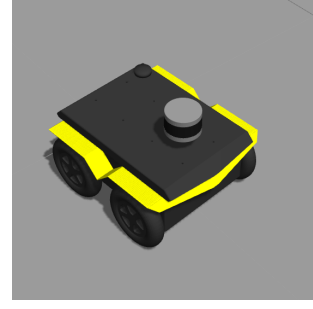
Fig. 4: Gazebo simulation of Jackal robot with Velodyne VLP-16.
