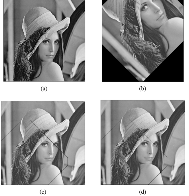
Fig. 5: The image registration results of two synthetic images. (a) is reference image r(x, y) and (b) is image s(x, y) . (c) and (d) are results of FMI and iFMI algorithm respectively.
